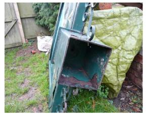
Here you can see the terrible condition of the base of the sign which secures it over the wooden post, it is rotten and rusted.
